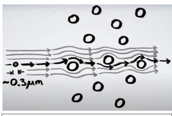
Figure 3: Motion of  $\approx 0.3 \mu m$  particles around uncharged fibres
